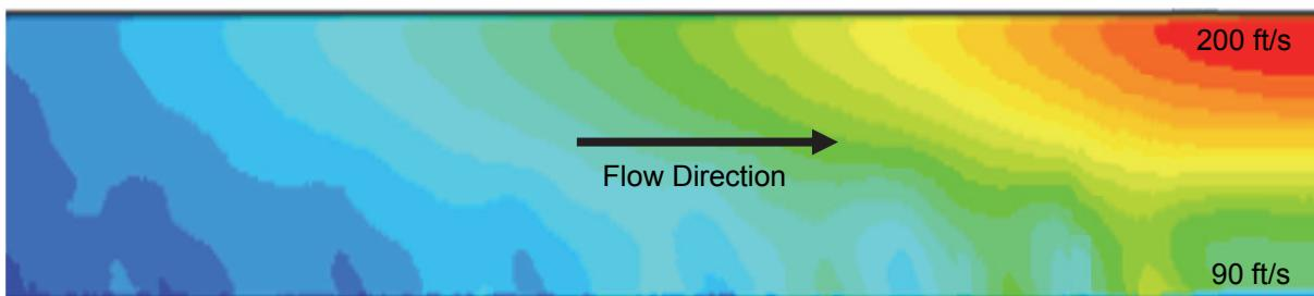
Fig. 8: Excessive Velocity near Top of Tunnel
