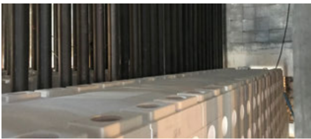
Figure 2. StaBloxTM reformer flue gas tunnel system.
