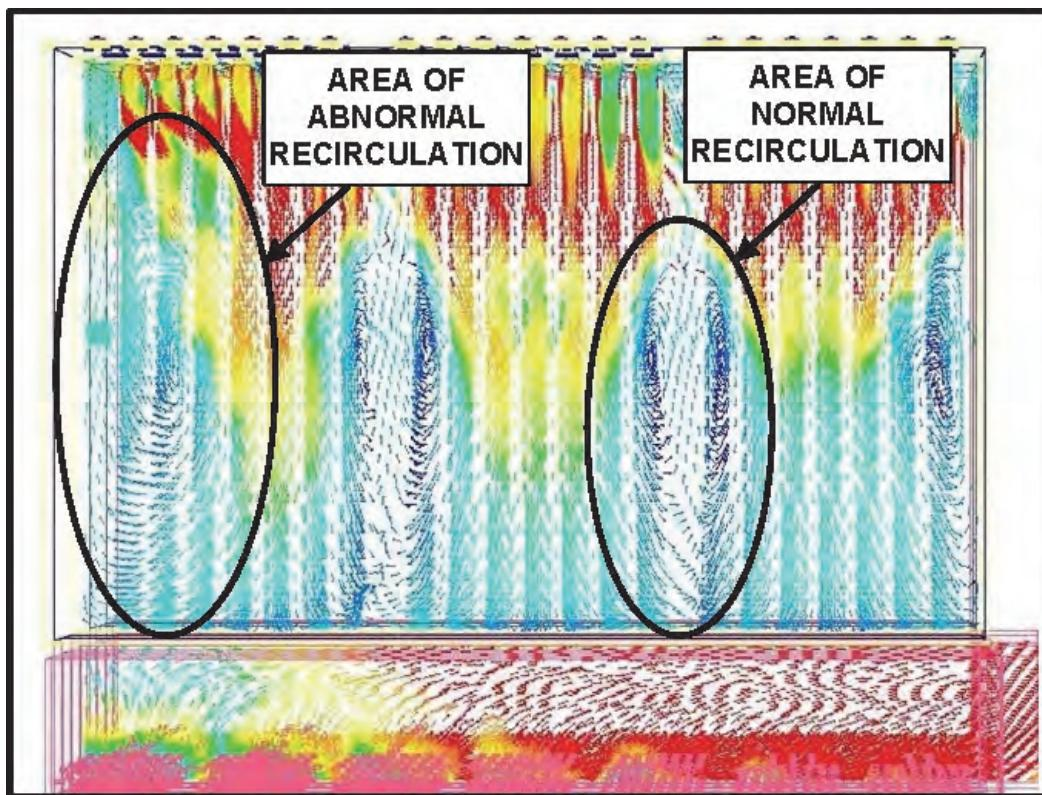
**Fig. 4: Flue Gas recirculation Patterns**
