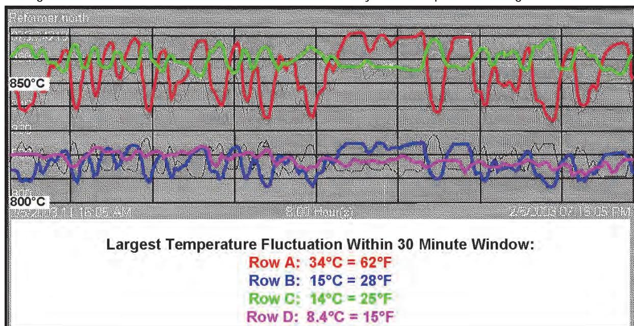
**Fig. 1: Process Outlet Temperature Fluctuations in a Methanol Reformer**
