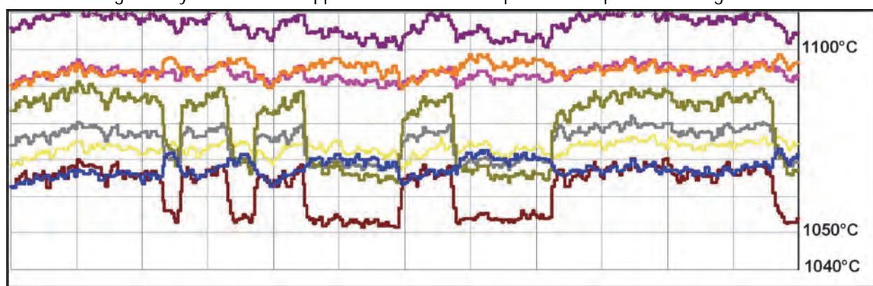
**Fig. 3: Tunnel Flue Gas Outlet Temperatures Corresponding to Figure 2**
