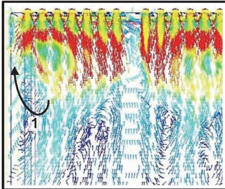
Fig. 6: Recirculation Pattern in Burner Row Plane
