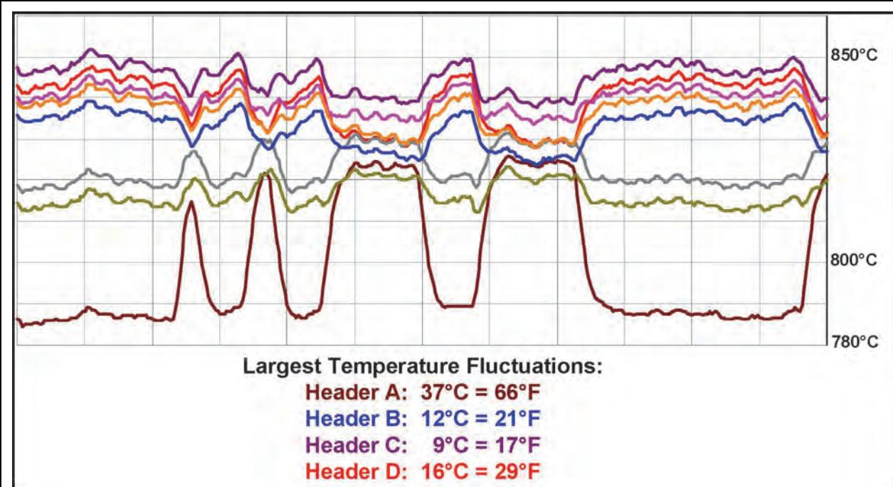
**Fig. 2: Process Outlet Temperature Fluctuations in a Hydrogen Reformer**
